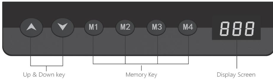
The whole handset surface is a button panel. If there is no press within 30 seconds, the screen is locked and M1/M2/M3/M4 keys are locked correspondingly, you should press Up or Down key first, it can be used when the display screen light up.
