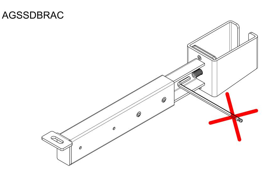
DO NOT TIGHTEN MIDDLE SET SCREW Failure to comply will void warranty
