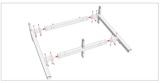
**STEP 2:** Assemble center legs and short rails together and fully tighten with provided screws.
