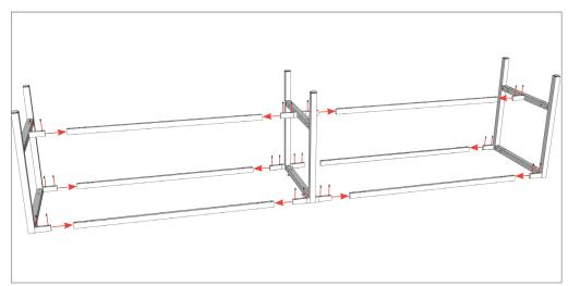
**STEP 3:** Assembly leg frames and long rails together and fully tighten with provided screws.
