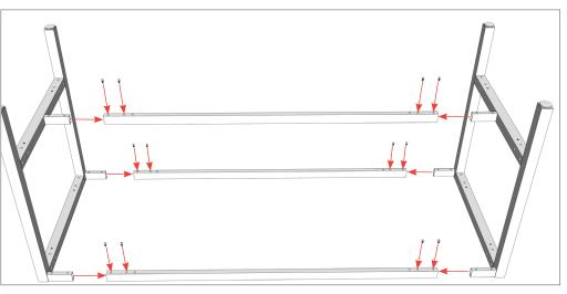
**STEP 2:** Assembly end leg frames and long rails together and fully tighten with provided screws.
