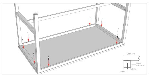
**STEP 3:** Pre-drill holes into the worktop, place worktop on a clean, flat surface and fully tighten the worktop to each rail using the provided screws.
