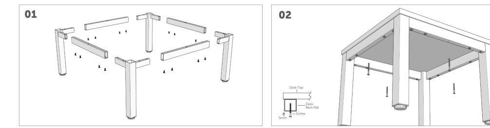
Assemble frames and rails together, loosely (1 turn from tight).
