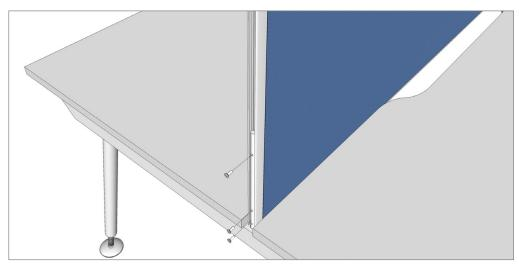
STEP 4: Slide centre screen pole over bracket. Carefully remove end seal on centre screens & fit screen between end brackets & screw self tappers to fix screen tightly.
