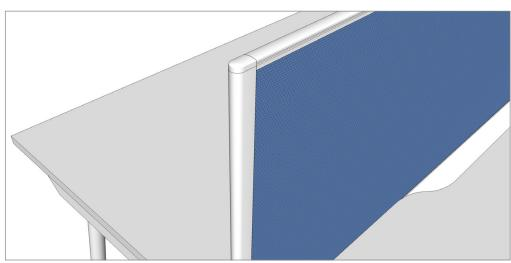
STEP 5 Attach centre screen end seal and top cap with soft non-marking mallet.
