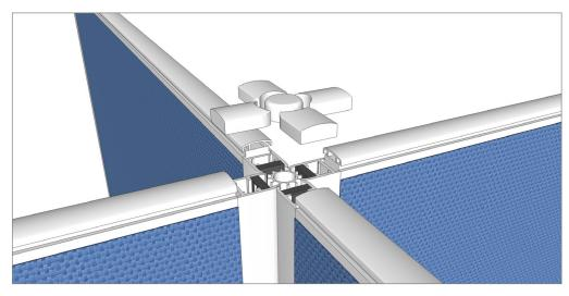
**STEP 11:** Install all top caps simultaneously down all together gently tapping with a soft non- marking mallet.
