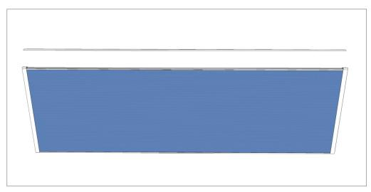
**STEP 12:** If for whatever reason you have to remove the top seal, then to refit, slightly arc in the middle, placing the 2 ends into location, & gently tap down.
