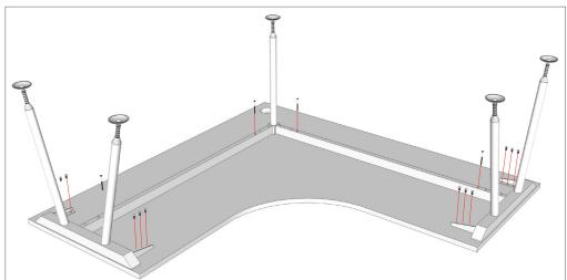
**STEP 2:** Fix desk top with 5mm overhang over metal frame. Lastly, fully tighten all rail to frame screws.
