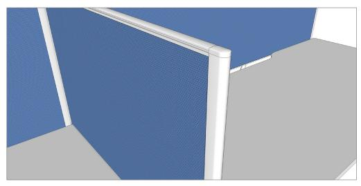
**STEP 10:** Attach return screen end seal and top cap with soft non-marking mallet.
