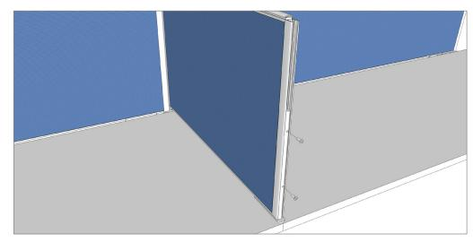
**STEP 9:** Remove return screen end seal, and attach screen to bracket with self tapper screws.
