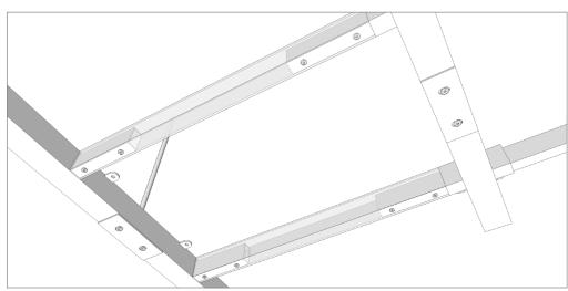
**STEP 13:** Fully tighten all rail to frame screws, & then screen bracket screws.
