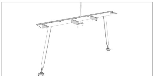
**STEP 2:** Assemble screen brackets to frame, loosely (1 turn from tight).
