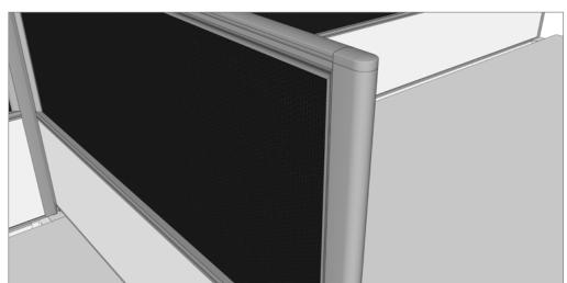
**STEP 10:** Attach return screen end seal and top cap with soft non-marking mallet.
