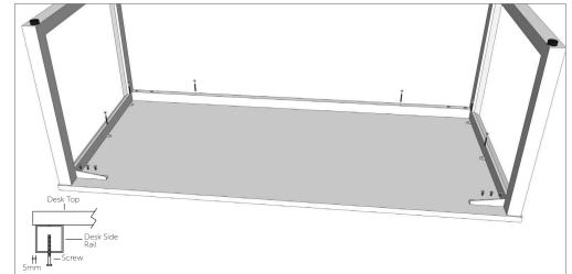
**STEP 2:** Fix desk top with 5mm overhang over metal frame. Lastly, fully tighten all rail to frame screws.
