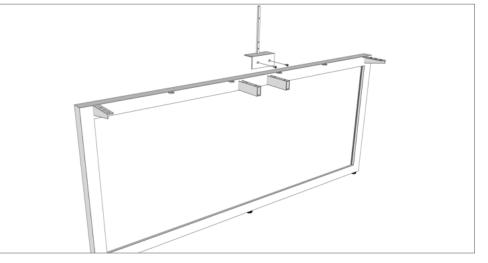
**STEP 2:** Assemble screen brackets to frame, loosely (1 turn from tight).
