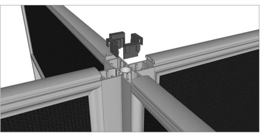
**STEP 6:** Attach screens to centre pole with top slug connectors.
