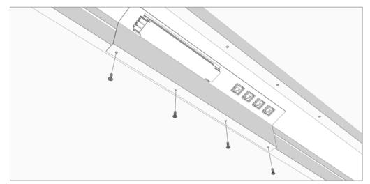
**STEP 13:** Fit power/data rails with screws into frame rail.
