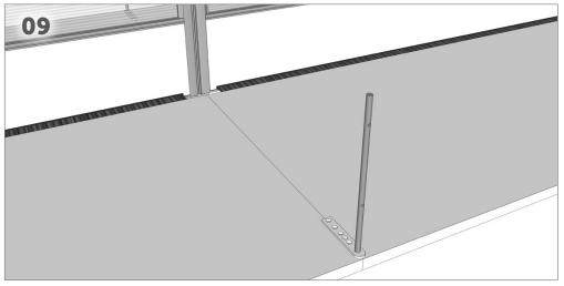
Remove return screen and fix bracket in place. As an alternative to screws, use 3M double sided tape to fasten return screen bracket to desk top.
