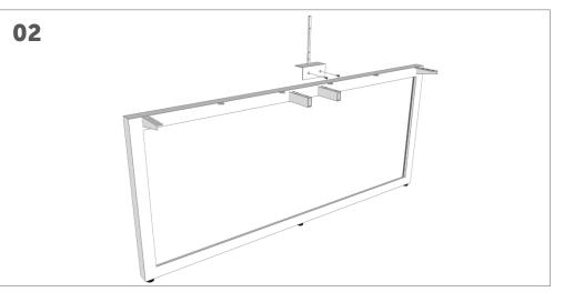
Assemble screen brackets to frame, loosely (1 turn from tight).
