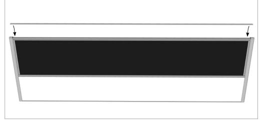
**STEP 12:** If for whatever reason you have to remove the top seal, then to refit, slightly arc in the middle, placing the 2 ends into location, & gently tap down.
