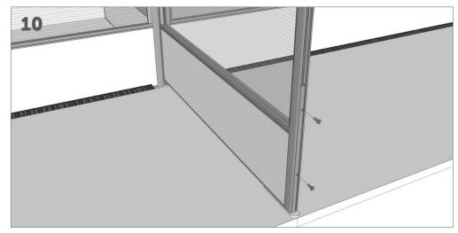
Remove return screen end seal, and attach screen to bracket with self tapper screws.
