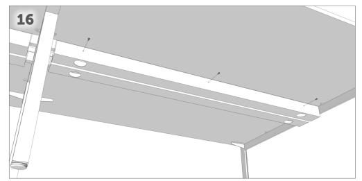
Attach cable trays with screws provided.
