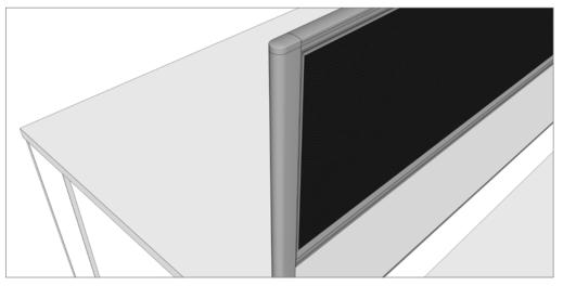
**STEP 5:** Attach centre screen end seal and top cap with soft non-marking mallet.
