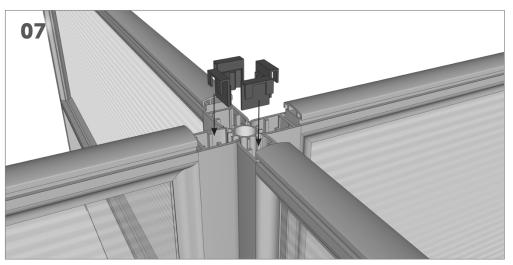
Attach screens to centre pole with top slug connectors.
