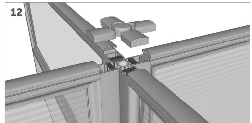
Install all top caps simultaneously down all together gently tapping with a soft nonmarking mallet.
