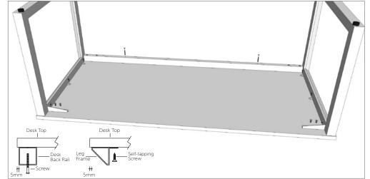
**STEP 2:** Fix desk frame to worktop, allowing for a 5mm overhang on all sides. Fully tighten all rail to frame screws.
