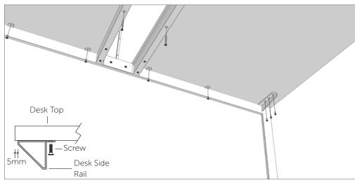
**STEP 3:** Fix desk top with 5mm overhang over metal frame. Where desktops butt together, make sure these are fitted tight together.
