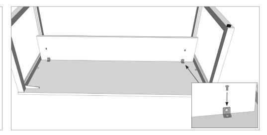
**STEP 4:** Pre-drill holes into the modesty and the worksurface, fully tighten with provided screws.
