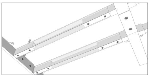
**STEP 14:** Fully tighten all rail to frame screws, & then screen bracket screws.
