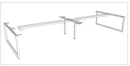
**STEP 1:** Assemble frames & rails together, loosely (1 turn from tight).
