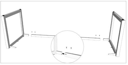
**STEP 1:** Loosely assemble frames & rails together (1 turn from tight).
