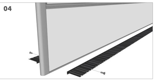
Screw fix the Comseal cable brushes to the base screen. Locate the correct height by resting the black Comseal extrusion against the top lip of the anodised bottom rail of the screen.
