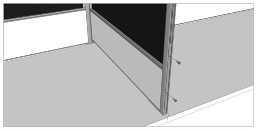
**STEP 9:** Remove return screen end seal, and attach screen to bracket with self tapper screws.
