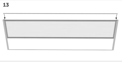
If for whatever reason you have to remove the top seal, then to refit, slightly arc in the middle, placing the 2 ends into location, & gently tap down.
