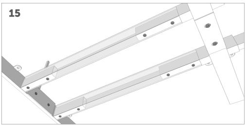
Fully tighten all rail to frame screws, & then screen bracket screws.
