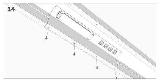
Fit power/data rails with screws into frame rail.
