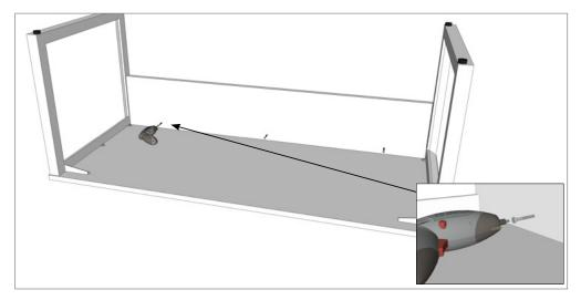
**STEP 4:** Pre-drill holes into the modesty and fully tighten the modesty to the rail with provided screws.
