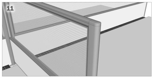
Attach return screen end seal and top cap with soft non-marking mallet.
