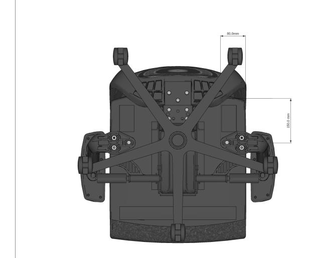
**STEP 1:** Measure 150mm from the back of the seat and 80mm from the edge of the seat to find the first hole.
