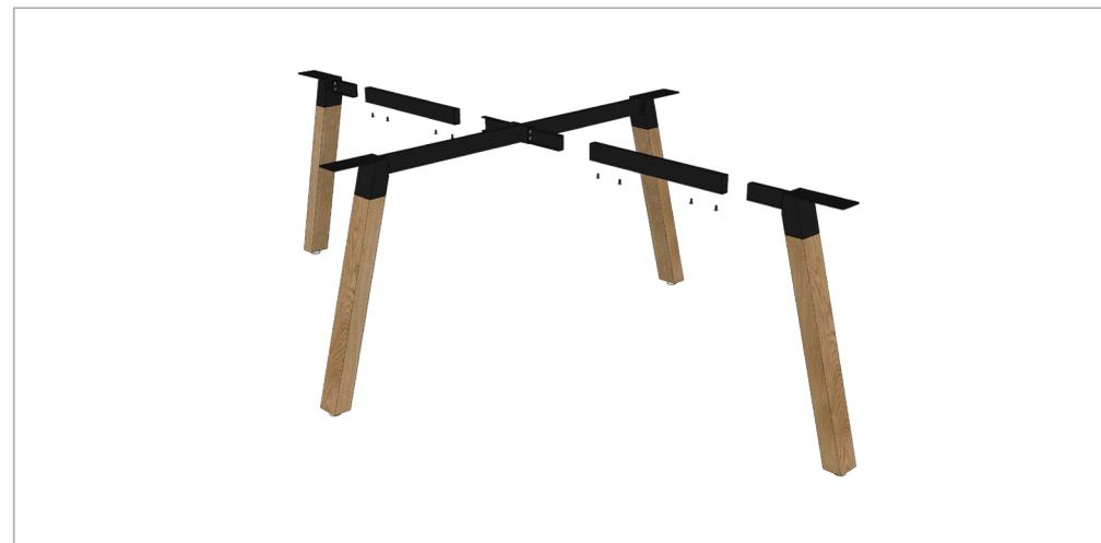
**STEP 2:** Connect centre rail, 2x short rails, 4 x legs together as shown.
