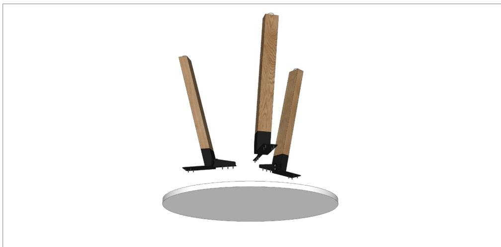
**STEP 3:** Fix the leg to the worktop using 4 x 23 mm self-tapping screws per leg.
