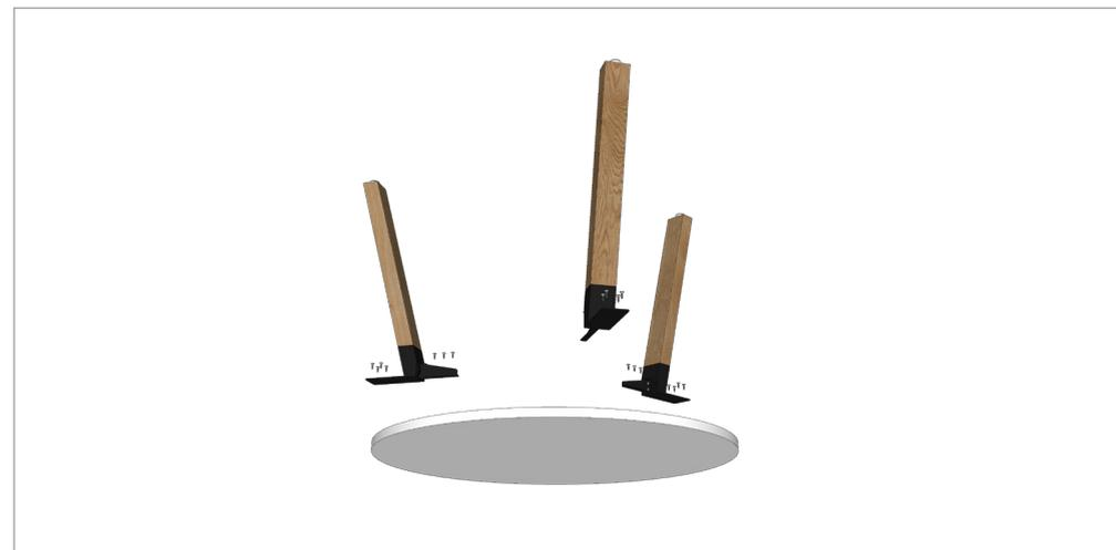
**STEP 2:** Align the legs at even spacing on the worktop, with the top plate being no closer than 5 mm from the edge of worktop. Mark each leg location for easy fixing in step 3.
