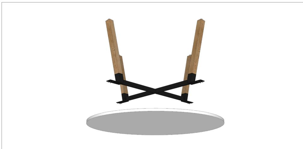
**STEP 3:** Align frame with worktop and fix down using 4 x 23 mm screws per leg and 4 x 70 mm screws for the rails.
