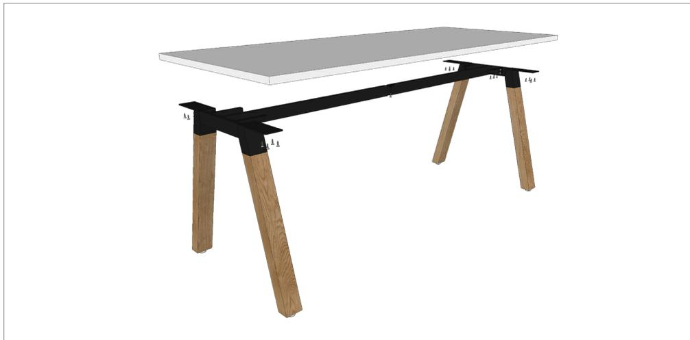
**STEP 3:** Align worktops to frame recommended spacing is 5 mm overhang on the ends.
