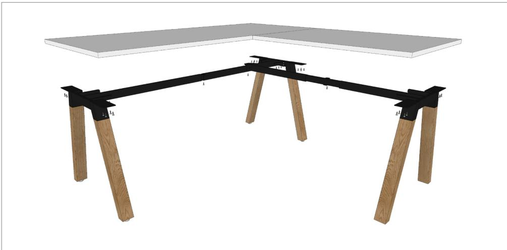
**STEP 3:** a.) Fit end leg to return top at 5mm off the end of worktop.
