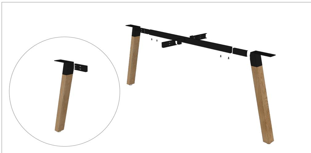
**STEP 1:** Fix 1x rail receiver to each leg using 2 x M12 bolts.
