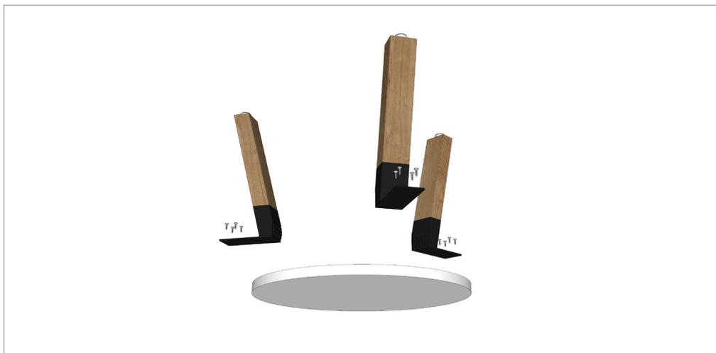
**STEP 1:** Align the legs at even spacing on the worktop, with the top plate being no closer than 5 mm from the edge of worktop. Mark each leg location for easy fixing in step 2.
