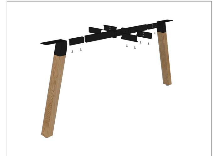
**STEP 3:** Assemble the mid leg using bolts provided in the spreader bar kit. Mount the rail to the centre mounting point.
