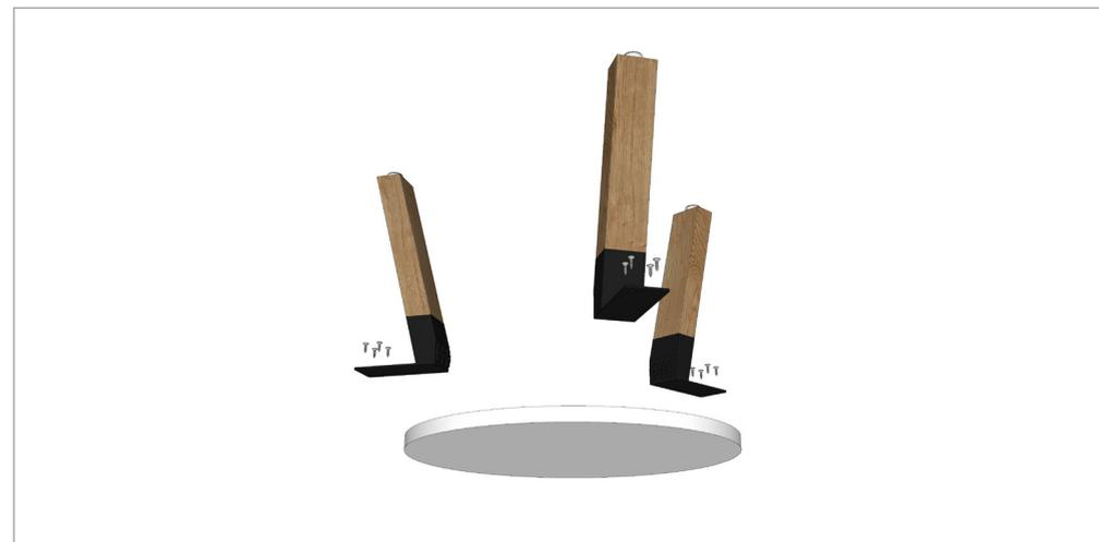
**STEP 2:** Fix the leg to the worktop using 4 x 23 mm self-tapping screws per leg.
