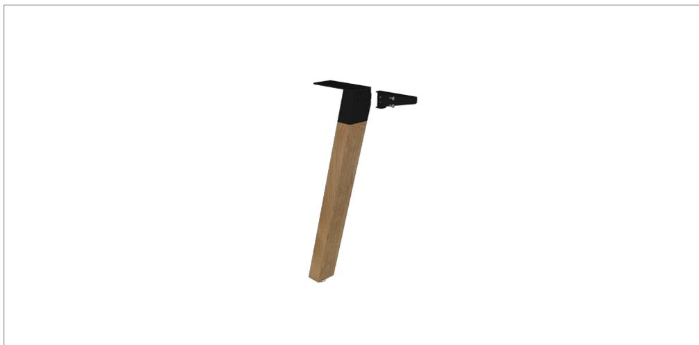
**STEP 1:** Fix 1x angle brack to each leg using 2 x M12 bolts.
