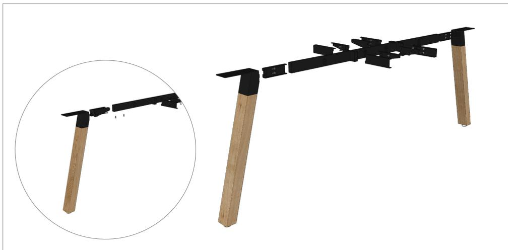
**STEP 1:** Assemble 1x mid leg set including assembling rail receivers to the crossbar.
