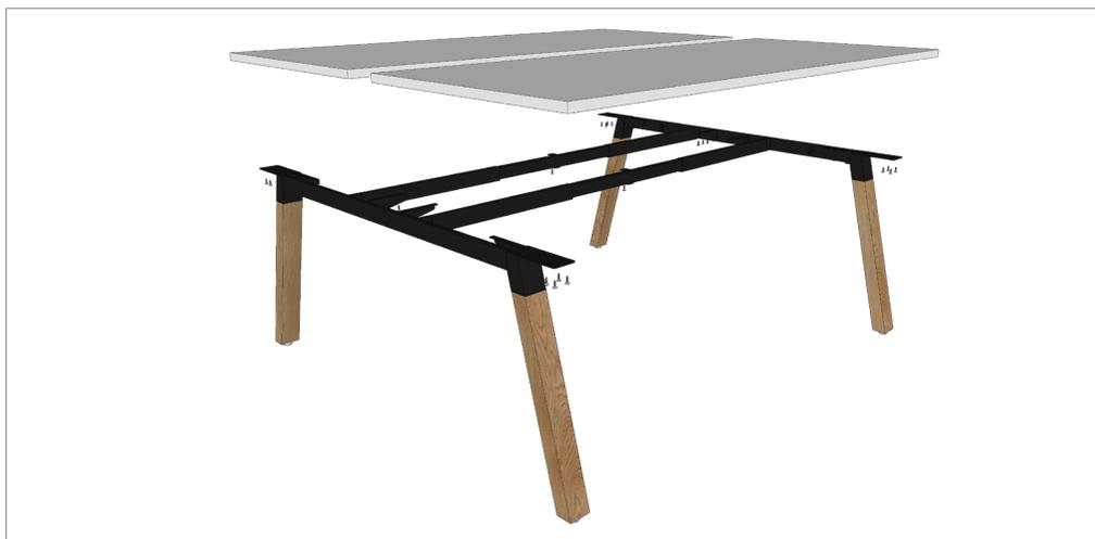
**STEP 3:** Align worktops to frame, recommended spacing is 5 mm overhang on the ends and central gap to suit screen type. (S50 = 52 mm, epanel = 20 mm, R18 = 20 mm)
