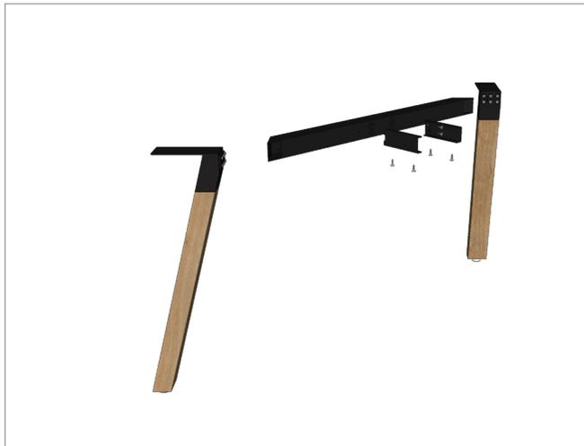
**STEP 1:** Assemble 2x end leg frames to the legs.
