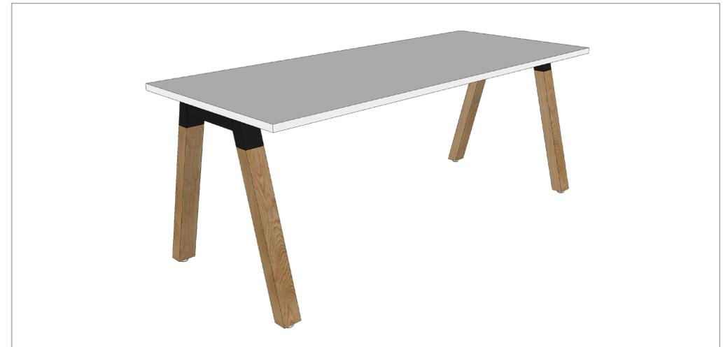
**STEP 4:** Fix worktop to frame using 4 x 23mm screw per leg, 2 x 23mm screw per rail.
