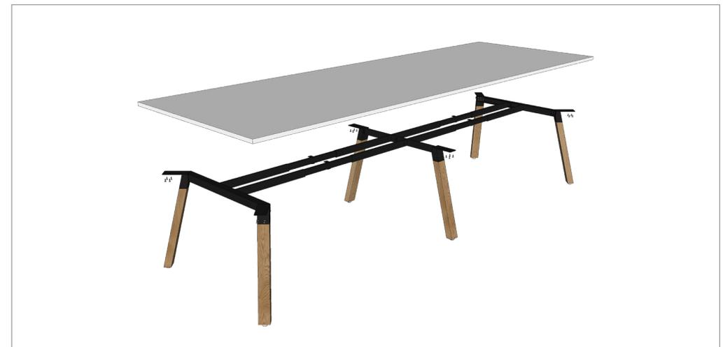
**STEP 5:** Fix worktop to frame using 4 x 23mm screw per leg, 1 x 23mm screw per rail.
