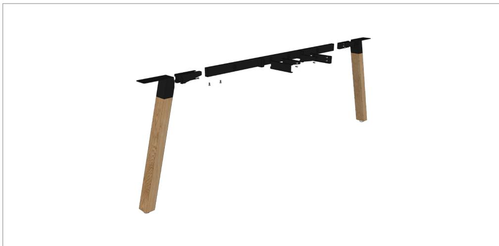
**STEP 1:** Assemble 2x end leg sets as above, including assembling the rail receivers to the crossbar.
