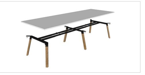
**STEP 5:** Fix worktop to frame using 4 x 23mm screw per leg, 1 x 23mm screw per rail.
