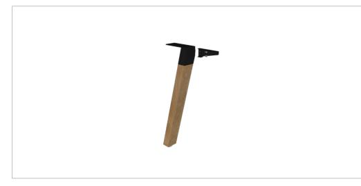
**STEP 1:** Fix 1x angle brack to each leg using 2 x M12 bolts.
