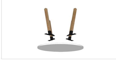
**STEP 3:** Fix the leg to the worktop using 4 x 23 mm self-tapping screws per leg.
