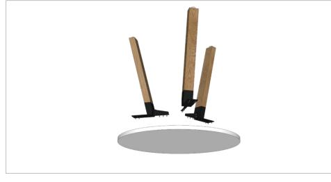
**STEP 3:** Fix the leg to the worktop using 4 x 23 mm self-tapping screws per leg.
