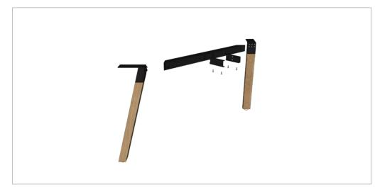
**STEP 1:** Assemble 2x end leg frames to the legs. Total 6 x M12 per leg.
