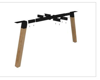
**STEP 3:** Assemble the mid leg using bolts provided in the spreader bar kit. Mount the rail to the centre mounting point.
