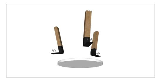
**STEP1:** Align the legs at even spacing on the worktop, with the top plate being no closer than 5 mm from the edge of worktop. Mark each leg location for easy fixing in step 2.
