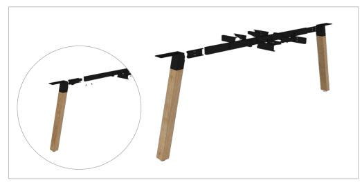
**STEP 1:** Assemble 1x mid leg set including assembling rail receivers to the crossbar.
