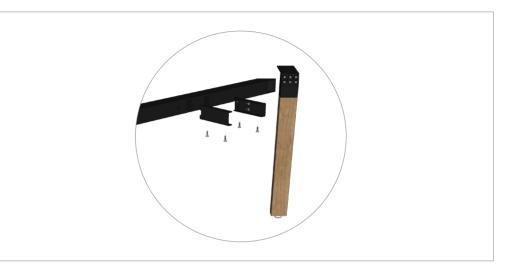
**STEP 2:** Assemble the rail receivers to the crossbar.
