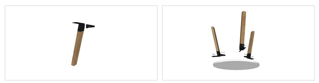
**STEP 1:** Fix 1x angle brack to each leg using 2 x M12 bolts.
