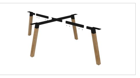
**STEP 2:** Connect centre rail, 2x short rails, 4 x legs together as shown.
