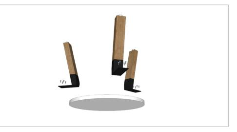
**STEP 2:** Fix the leg to the worktop using 4 x 23 mm self-tapping screws per leg.
