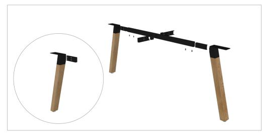
**STEP 1:** Fix 1x rail receiver to each leg using 2 x M12 bolts. Fix 2x rail receivers to the centre rail using 2 x M12 bolts.
