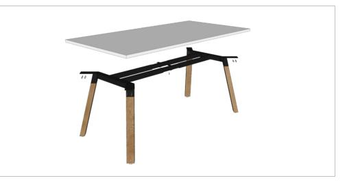
**STEP 4:** Fix worktop to frame using 4 x 23mm screw per leg, 1 x 23mm screw per rail.
