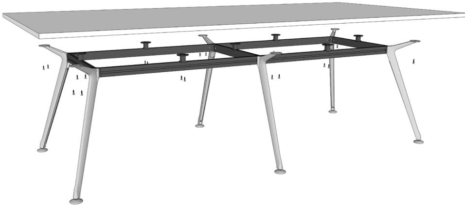
Ensure the work surface is centered over the frame. Pre-drill holes in the work surface. Fully tighten all M5x20mm self tapping screws through each leg and rail spacer bracket into the 25mm work surface.
