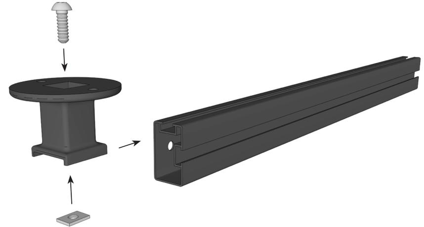
Loosely connect the longer M8x20mm dome head bolt and slot nut through the rail spacer bracket. Slide onto required rails and fully tighten in place. *800mm or longer rails require 1 bracket, 1600mm or longer rails require 2 brackets.*
