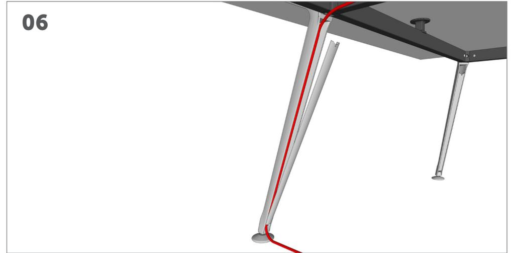
Conceal any power box cables using the magnetic leg cable covers.
