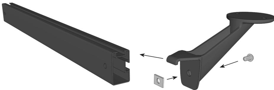
Loosely connect the shorter M8x12mm dome head bolt and slot nut through the metal rail spacer bracket. Slide onto required rails and fully tighten in place.
