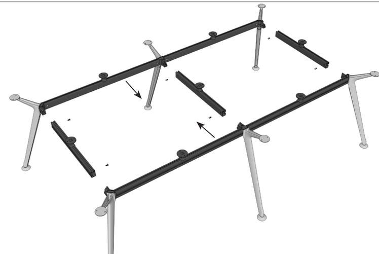
Securely connect legs to rails widths using the shorter M8x20mm dome head bolts.
