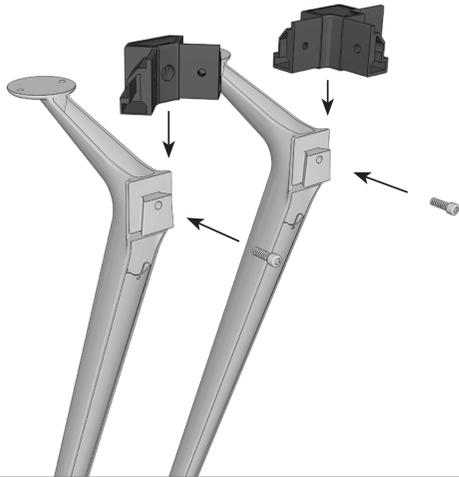
Slide the 2 way and 3 way connectors over each leg, and securely lock into place using M8x20mm cap head bolts.
