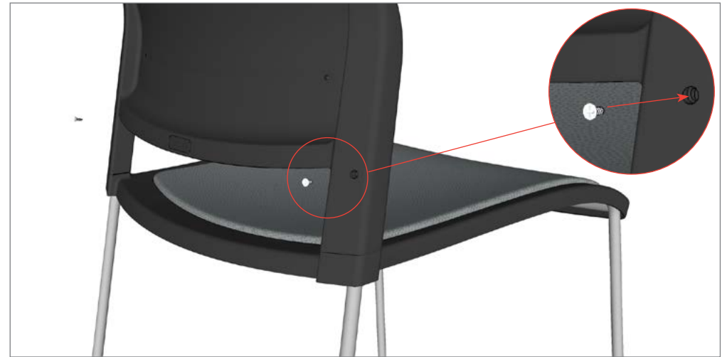
STEP 6: Fully tighten back shell to chair frame with provided screws.
