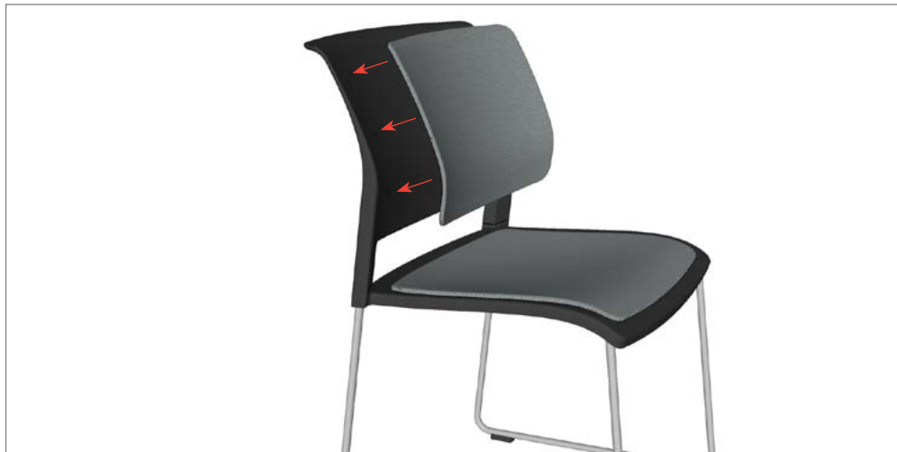
STEP 7: Mount back pad into back shell.
