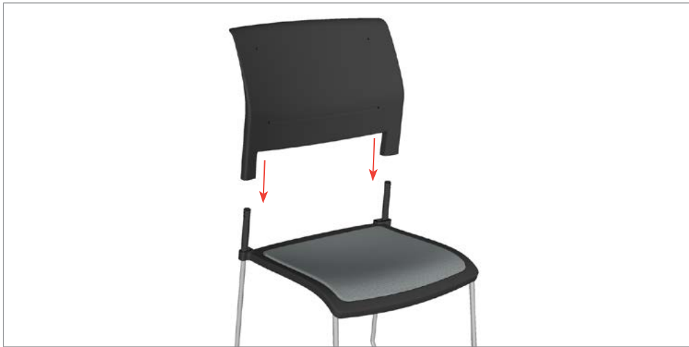
STEP 5: Silde back shell over chair frame.
