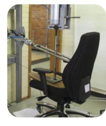
The testers examine the chair's ability to endure sporadic, static loads and evaluate its response to long-term use. The testers apply forces to the seat and back of chairs in load cycles of 50,000 repetitions. Chairs with Level 4 rating can endure 50,000 fatigue cycles, while those with Level 5 rating can withstand 100,000 cycles, and chairs rated Level 6 can sustain above 200,000 fatigue cycles
