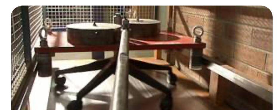
AFRDI also conducts impact tests to assess a chair's ability to withstand unexpected forces. They strike different points of the chair with a 6.5kg hammer to measure its impact resistance. The final impact test involves dropping the chair from a height such that it lands on a single leg.
