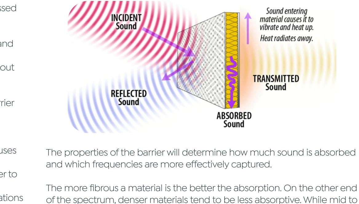
high-range frequencies are easily absorbed with standard acoustic treatment, low frequency sounds are very difficult to absorb because of d their long wavelength.
