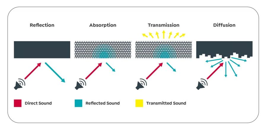
Essentially, when soundwaves strike an acoustic barrier, a portion of the sound is reflected, another portion is absorbed and converted into heat while the remainder is transmitted through the material.
