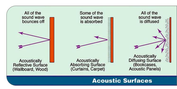
When it comes to acoustically treating any space, the idea is to use materials that both absorb sound and diffuse reflected sound to reduce the overall ambient volume..
